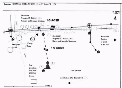
Mice Remarks: Off of pole 680642, build new single phase tap across CR 1170. Set (2) new primary poles, 25kva after, and short overhead service for temporary to build 4000kg house. Cost Due. Rue 1 Rev 1. Crews to clear branches in right-of-way if needed. Requires construction release. Hopkins County road crossing permit, and (2) easements. TLW
